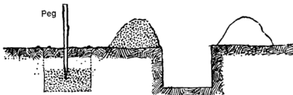
Soil from the top in one heap Soil from the bottom in another heap
